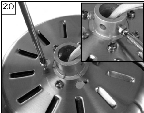
20 Remove 2 screws in yoke (see insert). Remove 3 screws with key-hole slots from top of fan.
